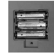
Insert 3 x AA batteries into the compartment ensuring they are installed the correct way around. The polarities are marked inside the battery compartment. Should the batteries have no polarity markings, the flat end of the battery should always be inserted against the spring. Reassemble the battery cover and tighten the screws to secure. Do not over tighten.
