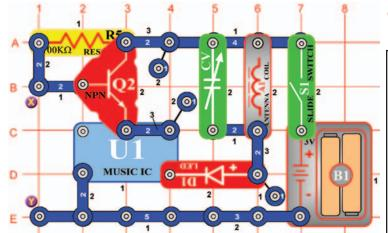
You need an AM radio for this project. Build the circuit on the left and turn on the slide switch (S1). Place it next to your AM radio and tune the radio frequency to where no other station is transmitting. Then, tune the adjustable capacitor (CV) until your music sounds best on the radio. Now connect a jumper wire between X and Y on the drawing, the music stops.
