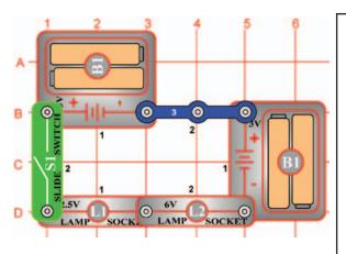
Turn on the slide switch (S1) and both lamps (L1 & L2) will light. If one of the bulbs is broken then neither will be on, because the lamps are in series. An example of this is the strings of small Christmas lights; if one bulb is damaged then the entire string does not work.
