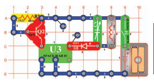
Place the circuit next to an AM radio. Tune the radio so no stations are heard and turn on the slide switch (S1). You should hear the space war sounds on the radio. The red LED (D1) should also be lit. Adjust the variable capacitor (CV) for the loudest signal.
