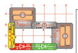
In this circuit the LED's (D1 & D2) will have the same brightness, but the lamp (L1) will be off. When connected in series, all components will have equal electric current through them. The lamp is off because it requires a higher current through the circuit to turn on than the LED's do.
