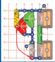
This light alarm circuit uses two transistors (Q1 & Q2) and both sets of batteries. Build the circuit with the jumper connected as shown, and turn it on. Nothing happens. Break the jumper connection and the lamp (L2) turns on. You could replace the jumper with a longer wire and run it across a doorway to signal an alarm when someone enters.
