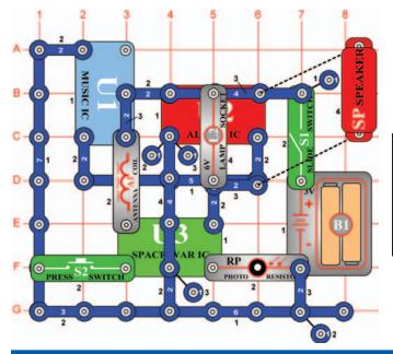
Build the circuit shown. Note that in some places parts are stacked on top of each other. Turn it on and press the press switch (S2) several times and wave your hand over the photoresistor (RP) to hear the full spectrum of sounds that this circuit can create. Have fun!
