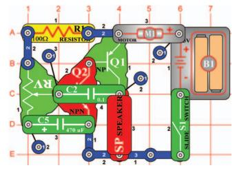
Build the circuit on the left. Turn on the slide switch (S1) and move the setting on the adjustable resistor (RV) across its range. You hear screaming sounds and the fan spins.
