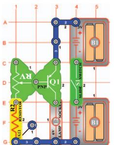
Build the circuit and vary the lamp (L2) brightness with the adjustable resistor (RV), it will be off for most of the resistor's range. The point on the PNP (Q1) that the lamp is connected to (point E4 on the base grid) is called the collector, hence the name for this project.
